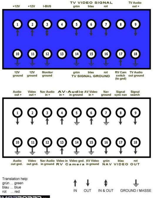
The 18 pin Blue comes from the car harness, to the TV, then you need the white plug to go from the video module with those pins I sent the wiring of to the Blue plug of the navigation computer. The blue pins
